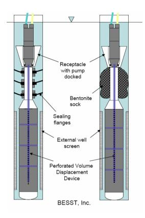
BESST's ZIST<sup>TM</sup> (patent pending) is the most economic and versatile system for isolating the well screen, eliminating drawdown, and reducina purae volume.
