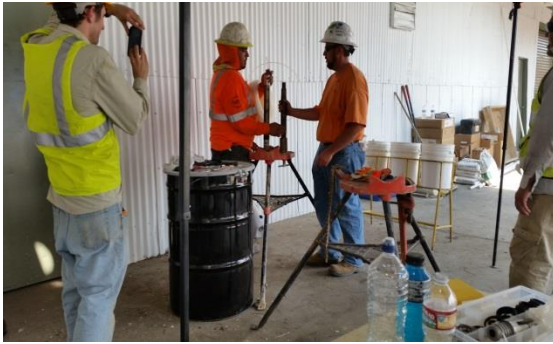
Figure 8: Attaching Mini Probe to Slotted AW Pin
