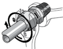
Figure 6: How to insert and tighten tubing into a tube connector.
