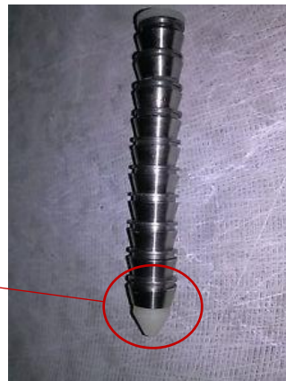
Figure 7: Stainless Steel Ferrules. There is a top and bottom to each ferrule set (Conical Top and Beveled Ringed Bottom). See circle
