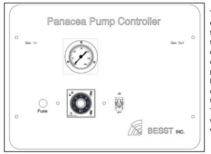
The TCU is housed in a sturdy Pelican case for increased portability and field durability, and features an easyto-use interface. A dual-cycle timer controls the discharge and recovery cycles times, and a pressure gauge provides a read out of the pressure being used. Timer controls are extremely flexible, allowing different times for discharge and recovery. This versatility enables use in a great variety of wells: low or high water volume, fast or slow recovery rates.
