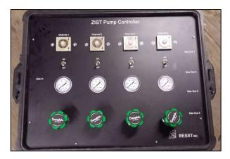
Figure 2- A 4-channel Timer Control Unit, used for nested or nearby wells
